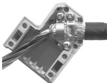
Figure 56: Connect the shield in the sub D connector
